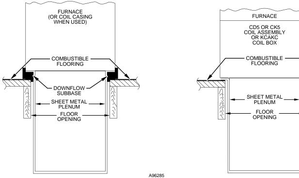
Fig. 6—Furnace, Plenum, and Subbase Installed on a Combustible Floor
