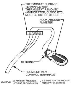
Fig. 20—Amp Draw Check With Ammeter A96316
