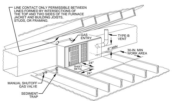
Fig. 8—Typical Attic Installation
