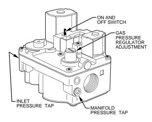
Fig. 18—Redundant Automatic Gas Control Valve
