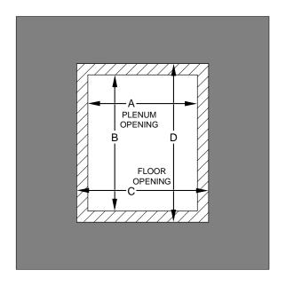
Fig. 5—Floor and Plenum Opening Dimensions
