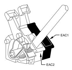
Fig. 16—EAC Terminals on Furnace Control
