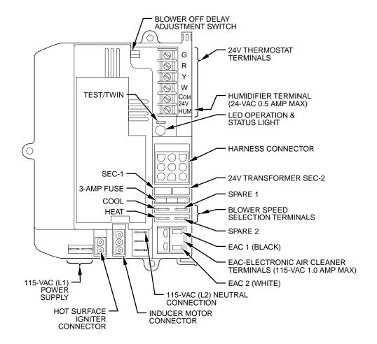
Fig. 14—Furnace Control
