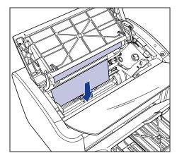
□ If the paper is difficult to pull out, pull on the leading edge of the paper as shown in the diagram ①, then remove the paper from the output tray side ②.
