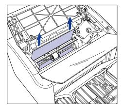
□ If the jam is difficult to clear, pull the paper out from the multi-purpose tray or manual feed tray.
