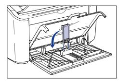
□ Slide the rear paper guide ① to align the small paper guide with the paper, and close the tray cover ②.
