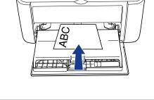
**3** Slide the paper guides to fit both sides of the index card.
