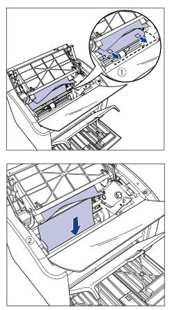
□ If the paper is difficult to pull out, pull on the leading edge of the paper as shown in the diagram ①, then remove the paper from the output tray side ②.
