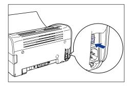
**2** Plug the supplied power cord securely into the power socket.
