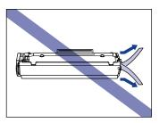
• Keep pulling on the tape until it is fully removed from the cartridge. If any sealing tape is left inside the toner cartridge, you may experience printing problems.
