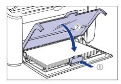
If you run out of paper and then refill the paper tray, the Paper Indicator will flash. Press the (Paper Key) to resume printing.
