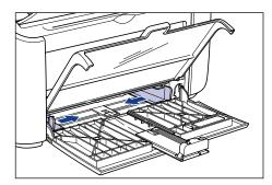
**3** Before loading transparencies or labels, fan them in small batches and align the edges.
