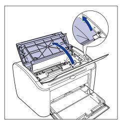
**2** Lift the toner cartridge in the direction of the arrows ①, then pull it out ②.
