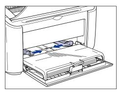
**2** Load the envelope with the printing surface facing up and the flaps closed and on the left side, then gently insert them all the way to the back of the tray.
