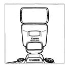
When the 420EX is mounted on a Type-A camera such as the EOS 30/ELAN 7E, using E-TTL autoflash is just as easy as normal autoexposure (AE). F-TTL autoflash uses the camera's multi-zone metering sensor for highly precise flash exposure control. A preflash is fired for evaluative flash metering and the reading is used to determine the main flash output. The result is a flash picture with excellent balance between the flash illumination and ambient light.
