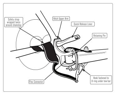
FIGURE 12: Forged hitch shown
