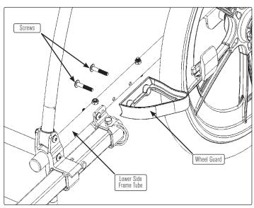
FIGURE 3: Wheel guard installation
