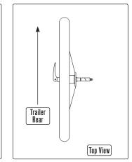
FIGURE 4: Quick release lever in unlocked "open" position
