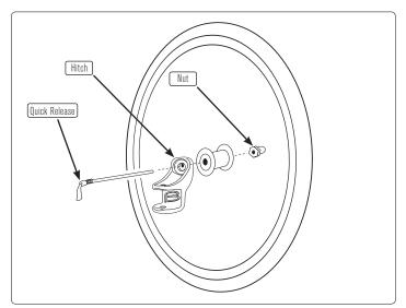
FIGURE 11: Quick release assembly
