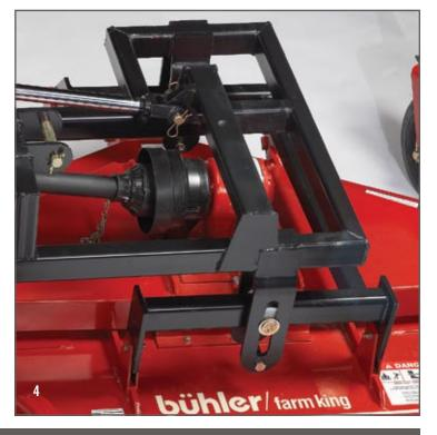
[1] The decks are lifted into position by hydraulic cylinders and are auto- [4] Heavy-duty decks and structural supports have solid reinforcing rods
