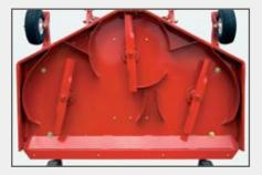
Each mower features three high-speed blades with one of the highest rated tip-speeds in the industry. This creates powerful suction that lifts the grass for a crisp cut. A blade overlap of 15%" to 25%" prevents stripping and ensures the lawn is mowed evenly.
