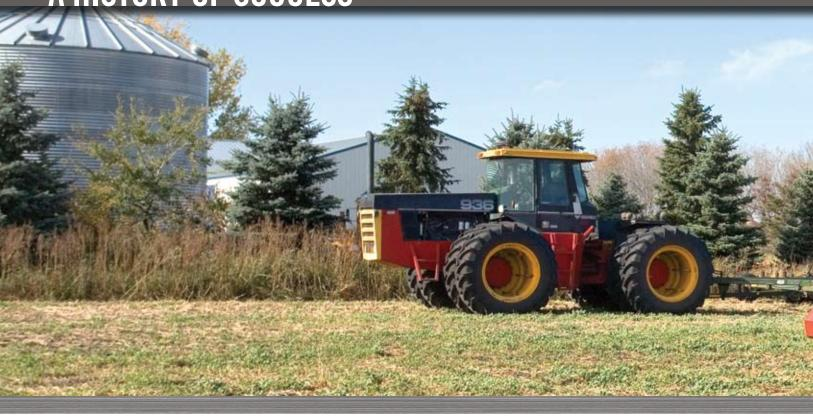
Versatile was the first company to massproduce articulated four-wheel drive tractors, starting in 1966 with the D100 and G100 four-wheel drives. Those ground-breaking tractors were primitive by modern standards, with a 6-cylinder diesel or 8-cylinder gas engine producing 100 horsepower. 1966 models sold for less than CA\$10,000.
