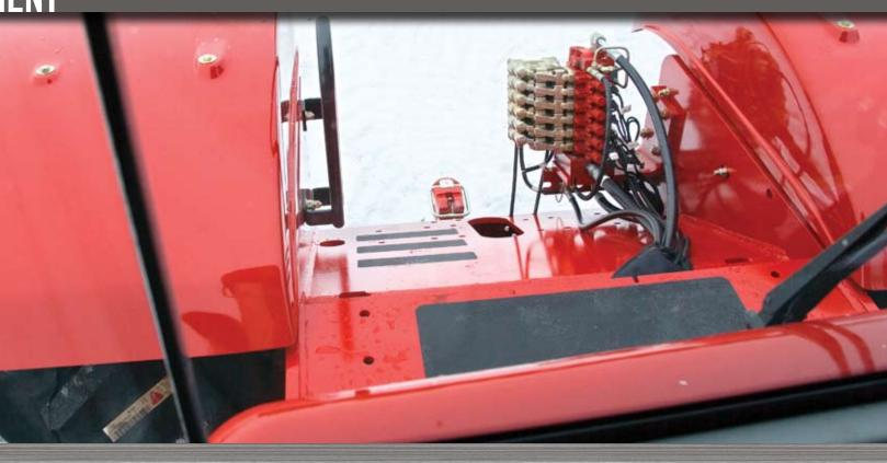
Optional electro-hydraulics are ergonomically designed for both comfort and convenience. Finger-tip controls manage the hydraulic functions and hydraulic flow is increased or decreased by rotary thumb wheels.
