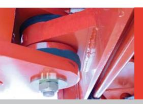
The drawbar pull point on Buhler Versatile four-wheel drives is immediately behind the articulation point, which now features a large-diameter pivot pin for maximum strength and durability. Models 305, 340, 375 and 400 feature a 2.36" (60 mm) pivot pin while the High Horsepower Tractor Series have a 3.15" (80 mm) pivot pin.
