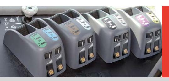
Electro-hydraulics are available and feature fingertip controls to manage the raise, lower, float and neutral functions. Each remote has a convenient thumb wheel for precise flow settings and programmable timed self-centering detents.
