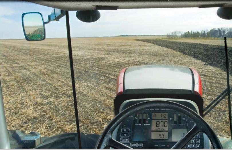
A mounting bracket and power center is available near the B-pillar for implement monitors, cell phones or GPS equipment.
