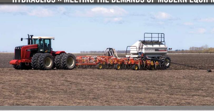
Modern implements require more hydraulic capacity to operate efficiently and the hydraulic system on Buhler four-wheel drive tractors has been developed to meet those demands. The closed center load sensing hydraulic system provides ample capacity for implements that demand high hydraulic flow by providing pressure and flow on demand. When no hydraulic power
