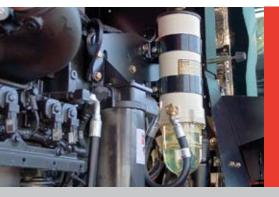
A large auxiliary fuel filter is standard equipment. With a larger capacity, the fuel filter ensures that fuel is thoroughly filtered to ensure harmful debris is removed before entering the engine, which is particularly important when using biofuels. This filter is visible from the ground or from the entry platform for easy inspection.
