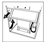
b. Remove second filter lying above blower. Slide filter toward rear of furnace and out of blower compartment. (See Fig. 15.)
