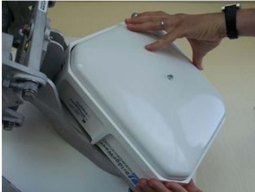
Figure 3-10 Attaching the radio to the back of the antenna
