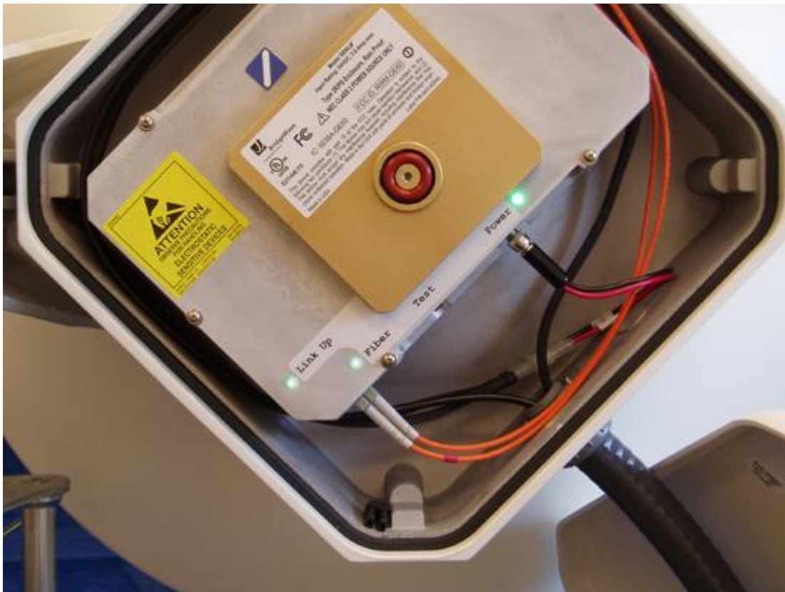
Figure 4-1: Link Up, Fiber and Power LED's indicating link is up and operating
