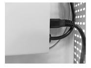
**Step 11:** Plug the trolley's mains lead in to a switched wall socket and switch ON. Switch on the unit's own ON/OFF switch located above the mains lead input.
