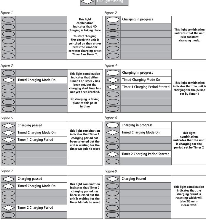
**NOTE:** If the time LED is not ON then NO charging is taking place. Unit needs to be turned ON to enable charging options to be selected.
