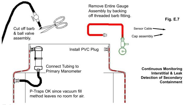
**E.4** - It is not uncommon for some interstitial fluid to be lost while connecting the tubing to the primary manometer. This is ok. Replace lost fluid by topping off manometer with interstitial fluid until the liquid level reaches just 2 inches below the top of manometer.
