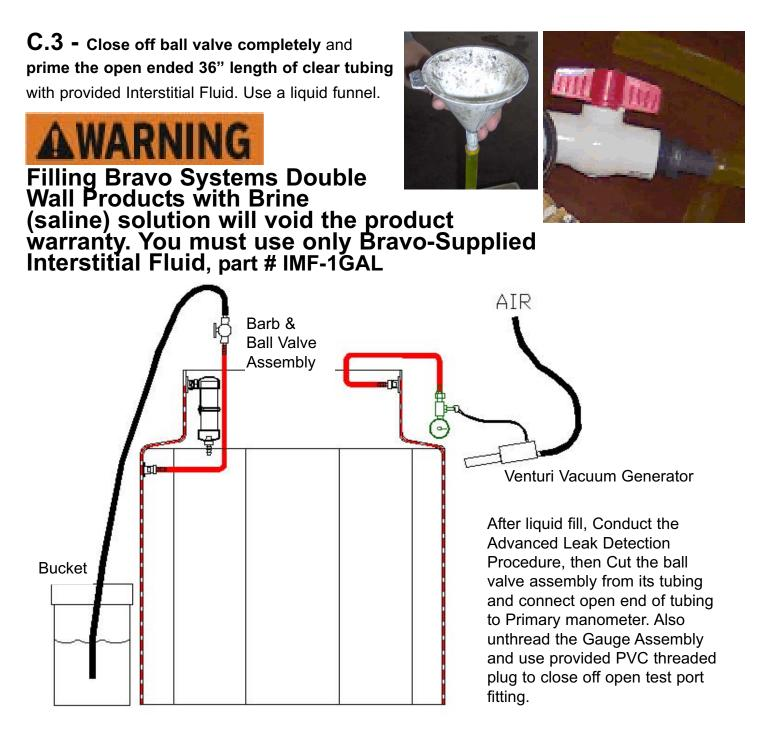
**C.4** - After filling the tubing all the way to the ball valve, **insert open end into your liquid source**. (5 gallon bucket filled with fluid is recommended.)
