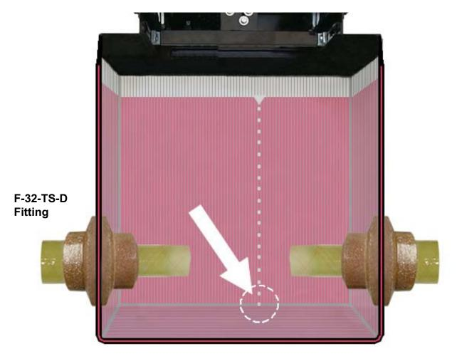
Here a leak is visible while a strong vacuum is pulled on the Interstitial space, forcing tiny air bubbles into the interstitial space to travel upwards. These streams of bubbles are easily spotted and can be traced down to its leak point or area.
