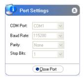
The Port Settings section displays the current used port settings for the connected BL-521 i.e. the port settings that were used to open and access the device. This includes the current COM port, Baud Rate, Parity and Stop Bits
