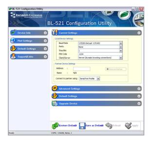
Add the address of your remote device into the "Partner Device Settings" Section in the "Address" field.
