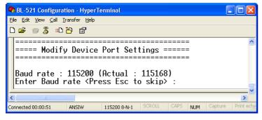
The user is first prompted to change the Baud Rate. The current setting is shown. To change the baud rate, just type the rate you want to use and press <enter>. The converter will accept any number you type, but will set the baud rate to the one that's closest to what it can actually achieve.
