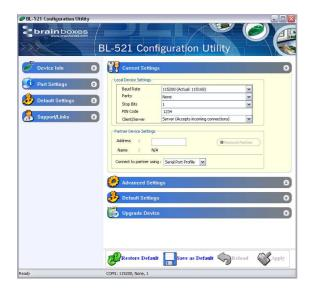
The Current Settings section is broken down into two sections; Local Device Settings and Partner Device Settings. Each field will be discussed further below.
