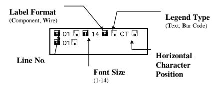
If you are entering more than 16 characters on a line, you will not be able to see the entire label until it is printed. The arrow keys allow you to move the cursor around the LCD. As the cursor moves beyond the 16<sup>th</sup> character, the screen will scroll to display the remaining text for
