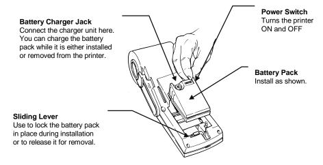
**NOTES:** The battery pack is shipped in an uncharged condition. Charge the battery for a minimum of 5 hours before operating the printer solely on battery power. You can charge the battery pack while the printer is turned "On" or "Off." The battery pack will be charging as long as the charger is plugged in.
