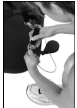
The squat cable feeds through the low pulley. The black plastic ball is on the side farthest away from the Power Rods.
