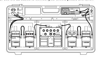
Connect the effects pedals with the 8pin parallel DC cable. Connect the L-shaped plug to DC OUT.
