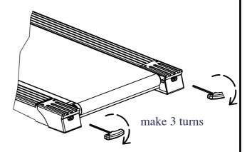
After assembly and before turning power on position the rear roller using the 'T' wrench (refer to the drawing if needed).
