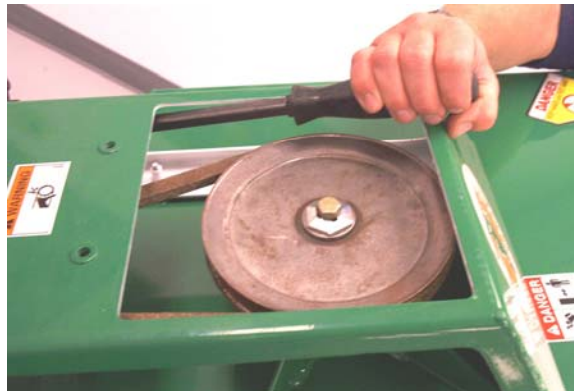
Adjusting Blade Drive Belt Tension
