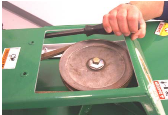
Adjusting Blade Drive Belt Tension
