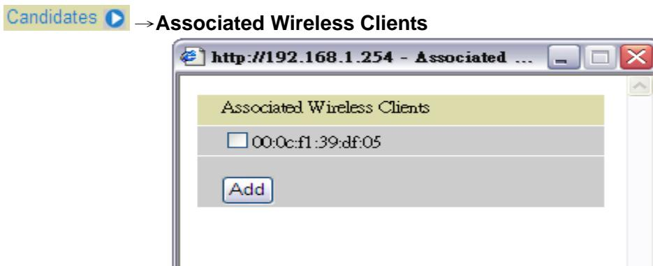
Associate Wireless Client displays a list of individual wireless device's MAC Address that currently connects to the router.
