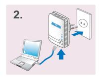
Create a secure network by a simply push off the network sync button.
