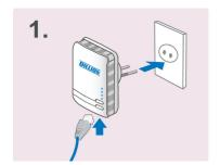
Then connect the BiPAC 2073 to a PC, modem, router or a set-top-box
