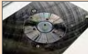
Guide bushing installed, centered and ready for template routing.
