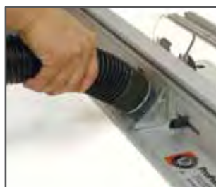
Built-in dust collection for 2-1/2" shop vac hose.
