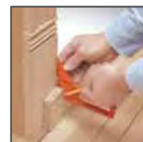
Notch allows you to align Trim-Loc with outside of trim and extend your line to the baseboard.
