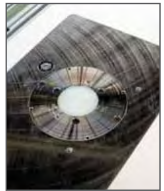
Zero clearance insert installed in a ProLift. Use when routing very small stock.
