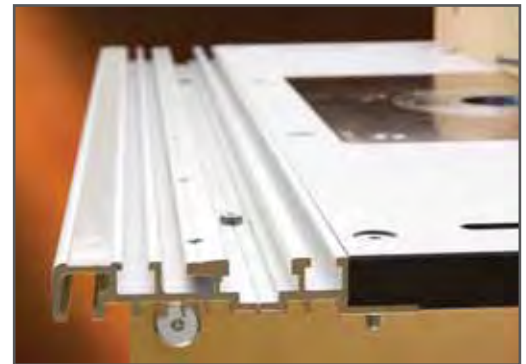
A row of hex-head set screws adjust the width of the miter track for a perfect no-slop fit.
