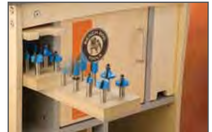
Pullout router bit trays provide easy access to your bits, keep them organized and ensure sharp, chip-free carbide.
