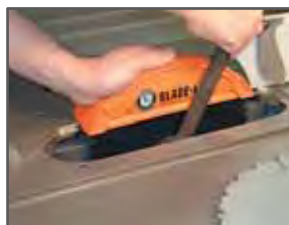
Place Blade-Loc over your blade and tighten.
