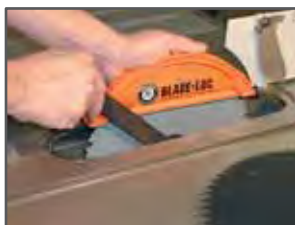
Place Blade-Loc over your blade and loosen the nut.
