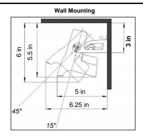
Remark: The bold-type values give the minimum distance required to be able to fully adjust the sensor.
