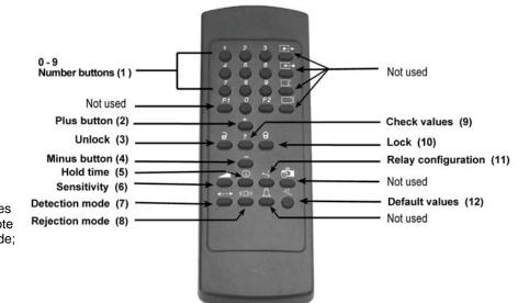
**Remark:** For optimum results point the remote control at the sensor before pressing its buttons.
