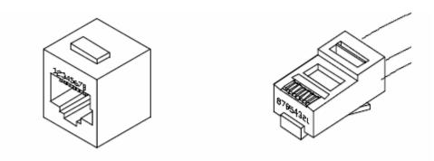
Fig. 1: RJ-45 Receptacle
