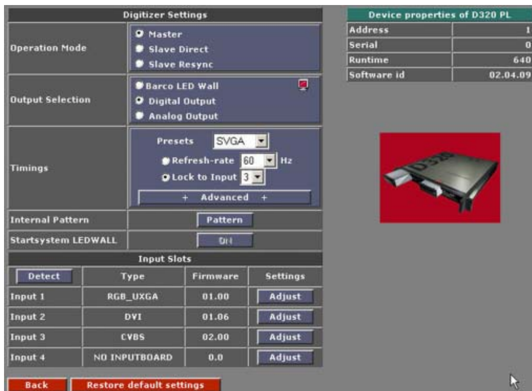
Image 10-1 Configuration window D320PL digitizer Digital or Analog output selected
