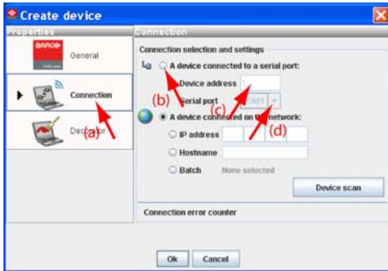
Image 5-5 Set up a serial connection
