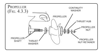
e. Coat the propeller shaft with an anti-seize lubricant (Figure 4.3.4).
