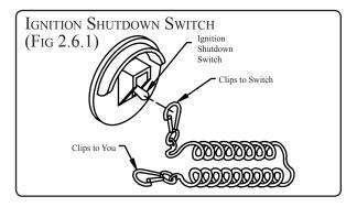
When the switch is used, the operator must securely clip the lanyard to their belt or clothing so that if the operator falls overboard or into the boat, the switch is activated and the engine shuts down. To reset ignition shutdown switch after it has been activated, simply reinstall the switch clip above the shut-off switch and flip the switch to the "UP" position.
