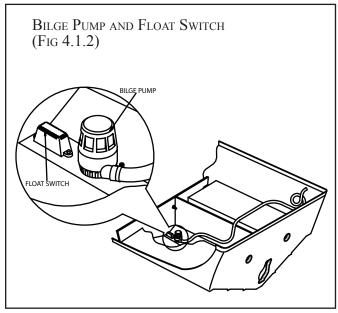
Before starting the engine, press the bilge pump switch so that the switch light comes ON. Make sure the pump is working by opening the engine compartment, listening to hear the pump running and check to see that liquid is being pumped out from the hull discharge. If the bilge has more liquid than normal, see Maintenance Section for locating and correcting the problem.
