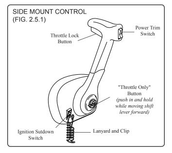
Shift/throttle controls are equipped with a "throttle only" mechanism which allows the shift mechanism to be to be disengaged from the throttle. This allows the throttle to be advanced without shifting the transmission when starting. It may be necessary to use the "throttle only" button in order to pump fuel into the engine for ease in starting.
