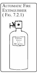
The indicator light, located on the dash, indicates to the helmsman when the unit has discharged. Under normal circumstances, the charge indicator light is lit. If the unit discharges, the light will go out.
