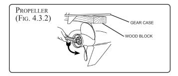
d. Remove the propeller nut retainer, the thrust hub and the continuity washer (Figure 4.3.3) and put them in a secure place. Pull the propeller straight off the shaft. Remove the thrust washer that is behind the propeller. If the propeller is seized to the shaft and cannot be removed by hand, special tools are needed. Have the propeller removed by an authorized dealer or trained mechanic.
