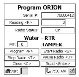
Starting the Badger ORION® Transmitter without the Programmer
