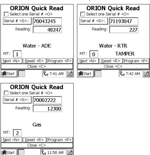
If you wish to monitor all of the readings that the Badger ORION<sup>®</sup> Receiver finds, clear the box next to Select One Serial Number by pressing the "O" key. When the RESET button "R" key is pressed, the Badger-Radix software will build a list of up to 50 received readings. Use the NEXT button "N" to view each of the readings in the list. When there are no more readings to display, the Badger-Radix will show this screen.
