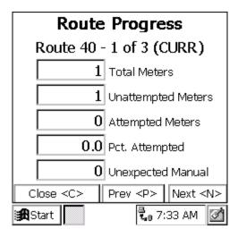
Use the N and P keys to view the progress screens for the next and previous routes loaded in the Badger-Radix. Notice that the route being displayed is the current route. If the route being displayed was not the one currently being read, you would see a screen like this.
