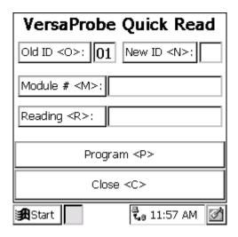
To start the read process for a VersaProbe, squeeze and release the trigger on the probe. The probe will read the module and forward the information to the Quick Read screen.
