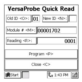
Once the data is correct, press the PROG button "P" on the Badger-Radix screen. **Note that the trigger button on the probe will NOT program the unit, but instead perform a quick read.** Once the programming operation is completed, you'll see the Successful message. If an error occurred, an error message will state the problem.
