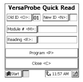
To program a Badger DIALOG module's reading and clear its tamper status, you must first get the specific information about that module. The easiest way to do that is to perform a Quick Read. Connect the VersaProbe<sup>TM</sup> to the Badger-Radix, place the sensor on the module, and squeeze and release the trigger on the probe. The probe will read the module and display the current status on the screen.
