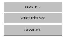
Choose the technology of the meter reading module. Choose VersaProbe "V" since that wand is the one used in Programming Badger DIALOG modules. You'll see this screen.
