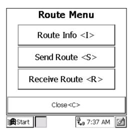
To load new meters into the Badger-Radix, press the Receive Route "R" key. To send meter readings back to Badger CONNECT, press the Send Route "S" key. Let's assume the Badger-Radix is sitting in the Loader-Charger and you wish to load a new route. When you press the "R" key, you'll see this screen.
