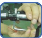
• Rotate hand brake assembly upward to a comfortable position then tighten bolt *(clockwise)* on the hand brake assembly with supplied allen wrench as shown.
