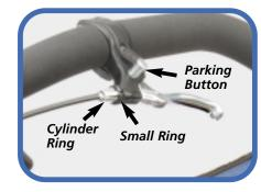
• If you don't have good braking action, simply squeeze the brake handle five or six times. If the problem persists, loosen the brake's cylinder ring to adjust the small ring, and then move the small ring away from the handle to tighten the cable. (Please do not over tighten!) To lock the rings, tighten the cylinder ring against the handle while holding the small ring in place.
