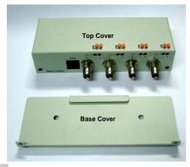
Step 5 Use the back cover as a template to mark the holes at the location required to mount the hubs.
