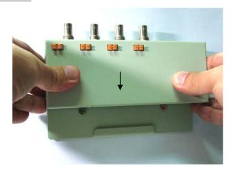
Step 8 Screw back the two countersunk screw to secure the top cover on to the back cover. Installation complete.
