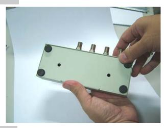
Step 3 Press slightly on the back cover using the left hand thumb and slide the back cover using the right hand.
