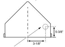
**NOTE**: a 3-1/2" diameter hole is required to provide clearance for the electrical inlet screws.
