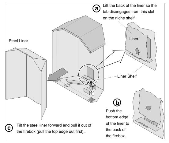
3 Install the liner following the directions below.
