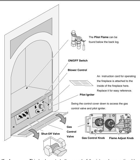
**Blower Knob** This knob controls the speed of the internal convection blower that
