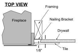
**NOTE:** When installed, there must be a minimum 1/8" gap between the face and facing.
