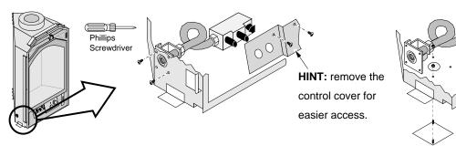
Position the gas inlet assembly over the hole in the baseplate (do not secure at this time).
