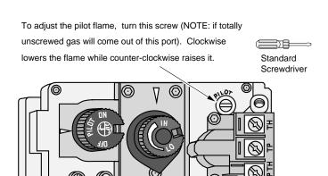
The pilot flame must contact the thermocouple and thermopile (see the illustration below). Adjust the pilot up or down as necessary.
