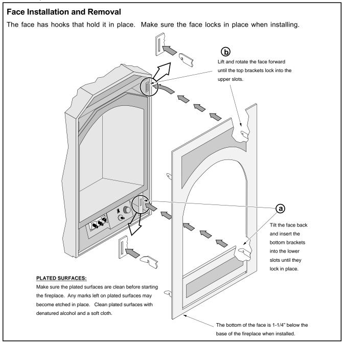
ACID WASH WARNING: Before installing the faceplate, make sure any masonry that has been treated with acid wash has been properly neutralized (this is used primarily with brick faces). Acid wash (muriatic acid) is used to remove excess mortar. If not properly neutralized with an ammonia solution, the gold face may develop a permanent tarnish when the acid evaporates over time. Contact your dealer if uncertain your facing has been properly neutralized.
