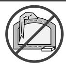
Do not place clothing or other flammable items on or near the heater. Because this heater can be controlled by a thermostat there is a possibility of the heater turning on and igniting any items placed on or near it.
