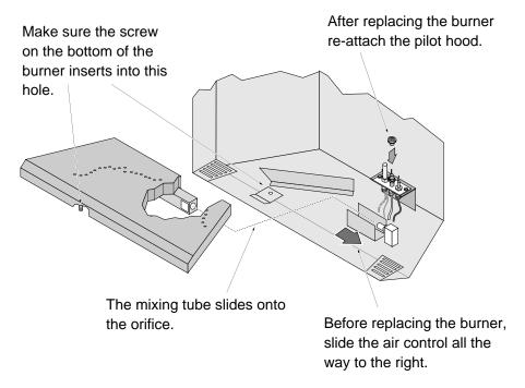
Make sure the burner is fully seated and pilot hood lines up with the burner holes at the rear edge of theburner.
