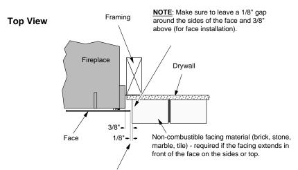
NOTE: When installed, there must be a minimum 1/8" gap between the face and facing.
