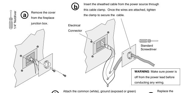
wires, and hot (black) wires from the power source to the
