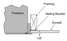
**NOTE:** When installed, there must be a minimum 1/8" gap between the face and facing.
