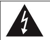
The Lightning flash and arrow head within the triangle is a warning sign alerting you of "dangerous voltage" inside the product.
