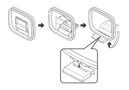
Press and hold the tab to insert the AM loop antenna lead wires into the AM ANT and GND terminals.
