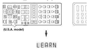
6 Press and hold the button you want to program on the other remote control until OK appears in the display window.
