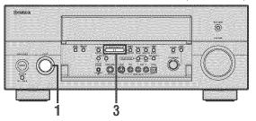
1 Rotate the INPUT selector (or set AMP/ SOURCE/TV to SOURCE and then press XM on the remote control) to select XM as the input source.
