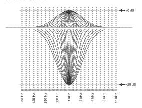
YPAO adjusts frequency characteristics to suit your listening requirements using a combination of the above three parameters (Frequency, Gain and Q factor) for each equalizer band in this unit's parametric equalizer. This unit has 7 equalizer bands for each channel.
