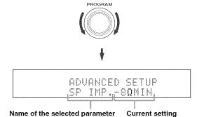
4 Press STRAIGHT (EFFECT) on the front panel repeatedly to change the setting.
