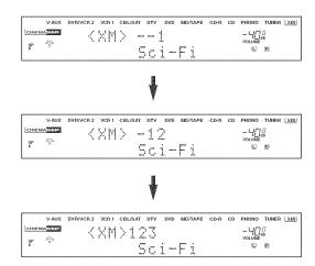
4 If you enter fewer than three numbers, you may press ENT. to tune to the channel immediately or wait a few seconds to confirm the entered channel number.
