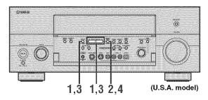
Select preset station E1 by using A/B/C/D/E and PRESET/TUNING/CH <1/▷.</p>
