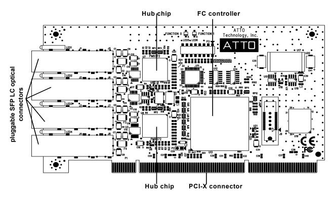
cannot connect both ports of a channel to an outside switch, you can connect one port to a switch and the other port to another device, thus daisy-chaining to make a public loop.
