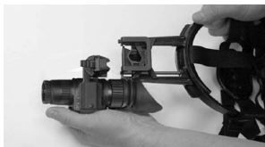
Figure 3-8 Attaching ATN NVM-14 to PVS-7 Headmount
