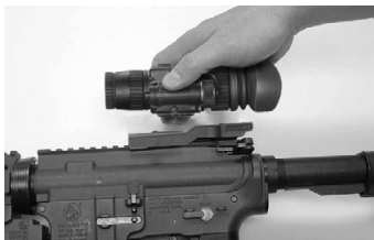
Figure 3-3 Attaching ATN NVM-14 to Weapon Mount
