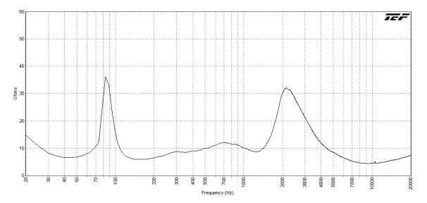
AH94-12ST Impedance (Ohms) vs. Frequency
