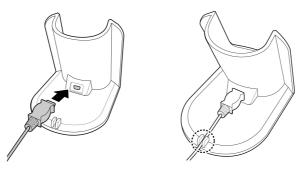
2. Plug the AC power adapter into the wall socket, and place your phone on the cradle for charging to begin.
