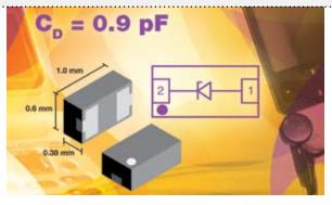
The VBUS051BD-HD1 from Vishay Semiconductors is an ESD, single line protection diode providing 0.9pF typical and 1.3pF maximum capacitance in the new LLP1006 package; its 0.6mm by 1.0mm footprint and ultra-low profile of 0.38mm saves board space. It is highly suited to ESD protection of portable electronics in mobile computing, mobile communication, consumer, industrial and medical applications.
