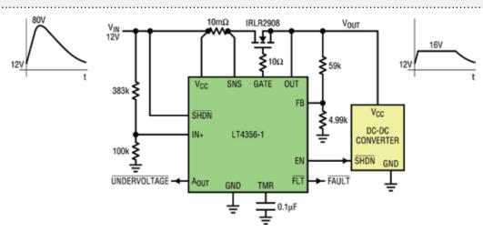
Even short duration, high voltage power spikes threaten the electronics in automotive and industrial applications although they may only last from a few µs to hundreds of ms. Critical electronic subsystems must survive these transients, rejecting surges, spikes and transients; in many applications, they must also operate reliably throughout such events.
