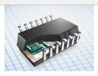
Infineon's KP 126 combines high precision with low cost in miniaturised SMD packaging. An integrated signal-conditioning circuit fabricated in BiCMOS technology performs the sensing function using a surface-micromachined array of capacitive sensors, amplifies the sensor cell output then compensates and linearises the temperature using a third order, polynomial transfer function. The resulting output voltage is proportional to the applied pressure.
