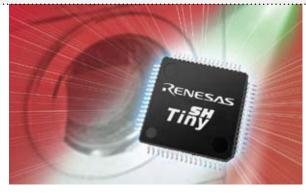
Low-end motor control applications require increasingly sophisticated control algorithms to squeeze improvements in energy efficiency from the new generation of motors. The SH/Tiny from Renesas is designed to meet these needs, and to bring design advantages when compared to standard digital signal processors.
