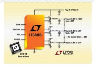
The LTC3853 is a highly efficient, synchronous step-down switching regulator, DC/DC controller with three outputs and numerous features that include output voltage tracking, Burst Mode<sup>®</sup> operation and pulse skipping, which safely powers pre-biased loads.
