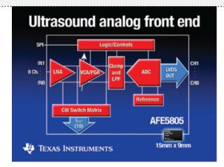
Texas Instruments' AFE58xx Analogue Front End (AFE) devices integrate multiple high-performance analogue circuits, providing superior image quality for a wide range of ultrasound applications. The devices consume less power and are more than 50% smaller than comparable devices in the market.
