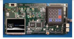
Blackfin ADSP-BF52x and ADSP-BF54x processors from Analog Devices are designed for use in performancedemanding portable products that require a wide range of connectivity options.
