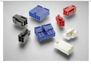
The VAL-U-LOK connector system from Tyco Electronics is a low cost, wire to wire, wire to board connector system with 4.2mm centreline spacing.
