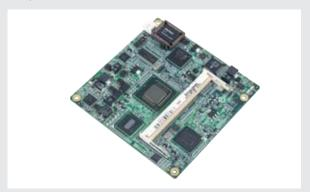
Figure 2: Advantech's SOM-6760 Micro Computer On Module
