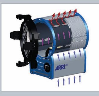
temperatures by 25%. Cross cooling allows ARRI TRUE BLUES to safely operate at almost any tilt angle.
