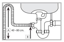
Before connecting the water outlet hose to the sink drain, remove the plastic plug (B).
