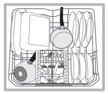
Very soiled dishes and pans should be placed in the lower rack because in this sector the water sprays are stronger and allow a higher washing performance. Several dishwasher models are fitted with tip-up sectors<sup>\*</sup>. They can be used in a vertical position when arranging dishes or in a horizontal position (lower) to load pans and salad bowls easily.
