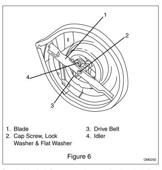
Check drive belt for wear or damage. Replace belt if worn or damaged.
