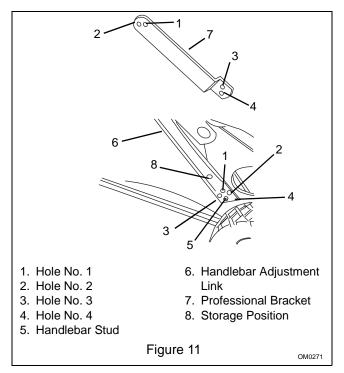
Use one of the four holes to adjust handlebar height to a safe, comfortable position. Place bolt on handlebar bracket through one of holes 1, 2, 3 or 4 in order of increasing height (See Figure 11).
