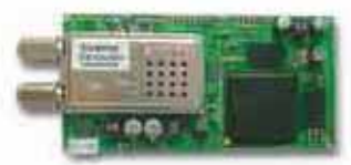
DTM-812 series In-vehicle high-definition DVB-T module, supports speeds of up to 230kph
