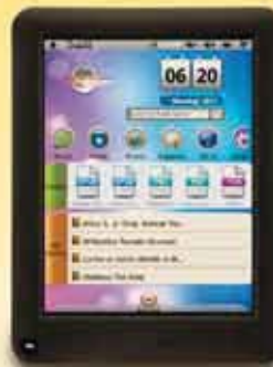
Smart e-book reader (T703) • 7" TFT-LCD resistive touch screen • Rockchip's RK2818 CPU • Google's Android 2.1 OS • Wi-Fi connectivity
