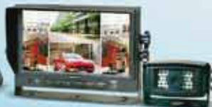
7" digital color TFT-LCD touch-screen monitor and weatherproof camera (MO-117D, CW-086)
