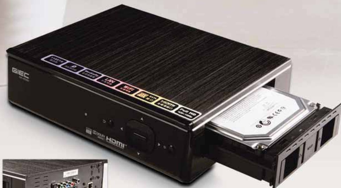
GK-HD260 HD multimedia player with Internet functions • Built-in 3.5" IDE SATA HDD • 1080p output • LAN and Wi-Fi connectivity
