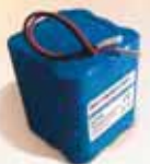
11.1V, 6.6Ah LiFePO 4 battery
