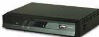
GK-B022SDB HD ISDB-T receiver, supports SBTVD-T, DVB, USB flash drive and MPEG-2 playback
