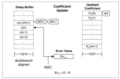
Figure 4-58 DIms\_2\_16x32 Coefficient update
