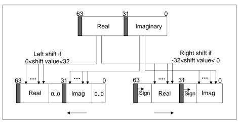
Figure 4-19 Complex number shift for 32 bits
