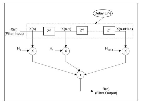
Figure 4-27 Block Diagram of the FIR Filter
