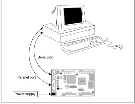
Figure 5-7 Hardware Setup
