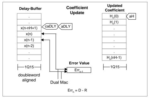
Figure 4-50 Dlms\_4\_16 Coefficient update
