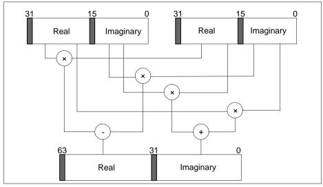
Figure 4-8 Complex number multiplication for 16 bits
