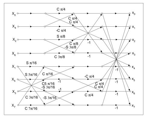
Figure 4-82 Signal Flow Graph for an 8-sample 1D IDCT
