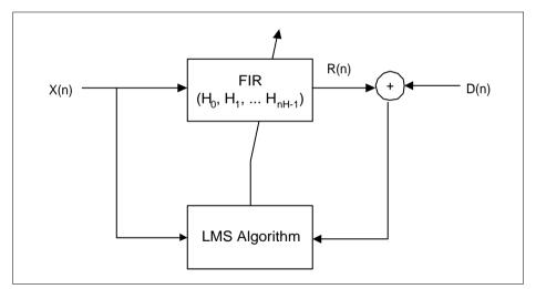
Figure 4-48 Adaptive filter with LMS algorithm
