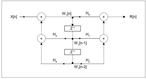
The block diagram for a biquad (second order) filter in canonical form is as follows.
