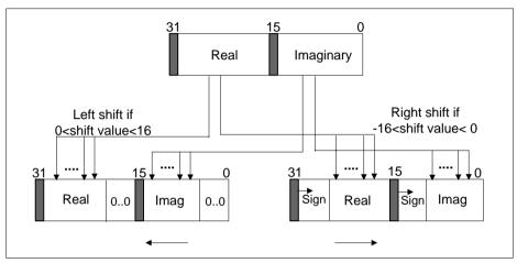
Figure 4-11 Complex number shift for 16 bits
