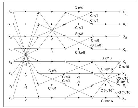
Figure 4-81 Signal Flow Graph for an 8-sample 1D DCT
