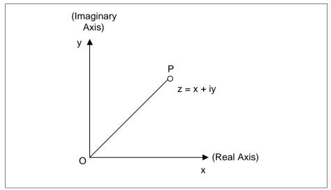
Figure 4-1 The Complex Plane (Argand Diagram)
