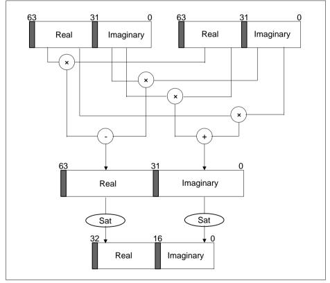
Figure 4-17 Complex number multiplication for 32 bits with saturation
