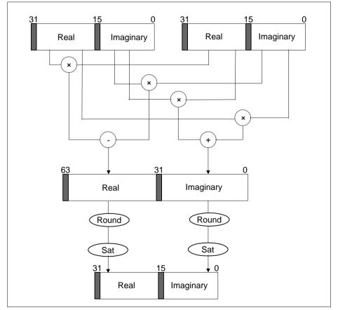
Figure 4-9 Complex number multiplication for 16 bits with saturation
