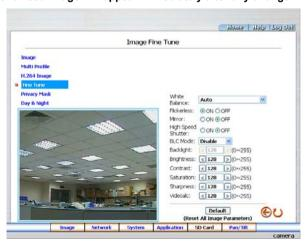
**NOTE:** The "videoalc" function only activates in connecting the auto iris lens (**DC IRIS**).
