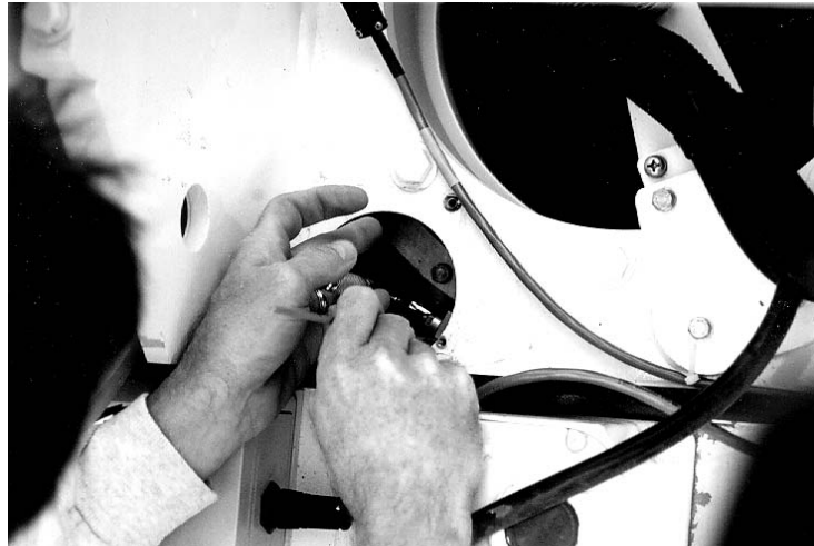
Figure 3. Adjusting Azimuth Cable Tension
