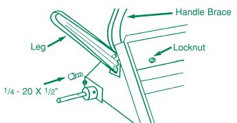
Remove spreader and components from carton. Place hopper on its front panel, insert two 1/4-20 X 1/2" hex head bolts through the leg; flattened end of handle brace and holes in hopper as shown. Install hex locknuts but do not tighten. Repeat on opposite side.
