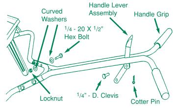
Stand spreader upright on wheels. Attach upper handle assembly to handle brace (make sure handle is positioned as shown) using four 1/4-20 X 1 1/2" hex bolts, eight curved wash-
