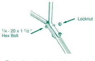
Install control tube between the control tube braces and secure with two 1/4-20 X 1 1/2" hex bolt and locknuts.
