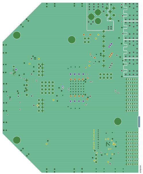
Figure 30. Evaluation Board Layout, Ground Plane (Layer 5)
