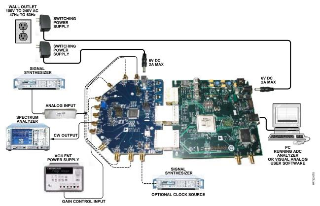
Figure 2. Evaluation Board Connection
