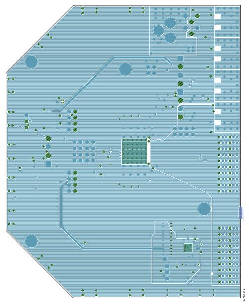
Figure 28. Evaluation Board Layout, Power Plane (Layer 3)
