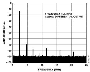
Figure 20. Typical Spectrum Analyzer Display of CWD Output
