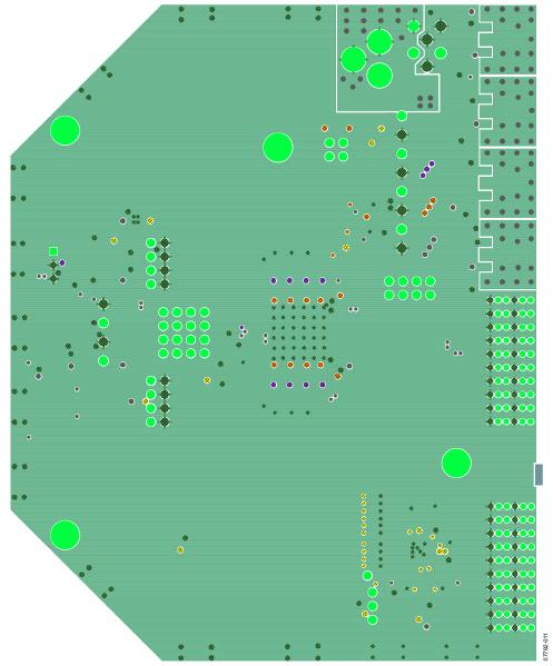
Figure 27. Evaluation Board Layout, Ground Plane (Layer 2)
