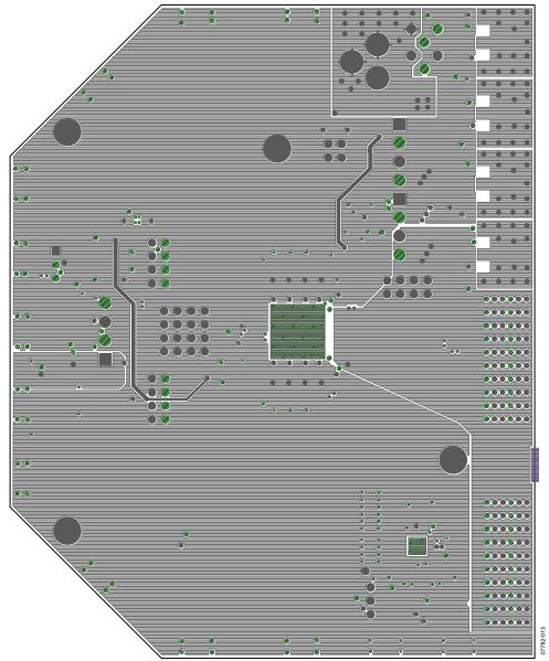
Figure 29. Evaluation Board Layout, Power Plane (Layer 4)
