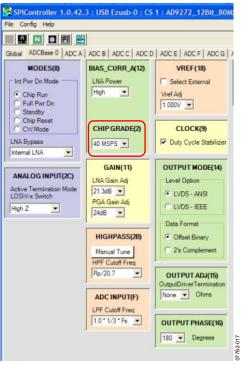
Figure 10. SPI Controller, CHIP GRADE(2) Box
