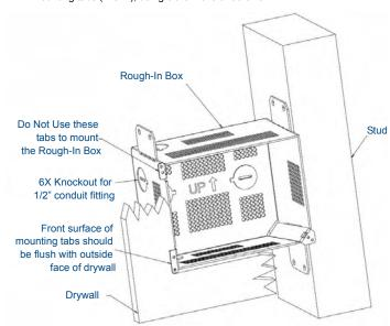
FIG. 1 CB-TP5 - Drywall Installation
