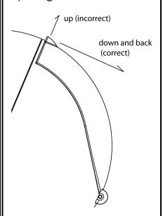
Do not attempt to open the hatch by using a fingernail to pull in an upward direction as this may break the latch mechanism.
