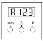
1. The Segment Display shows the DMX address of last change when powered this unit.
