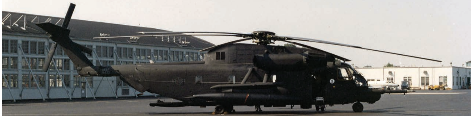
HH-53B # 66-14433, the "Black Knight," first Pave Low prototype. (Photo courtesy of Lt Col (ret) Frank Pehr.)
