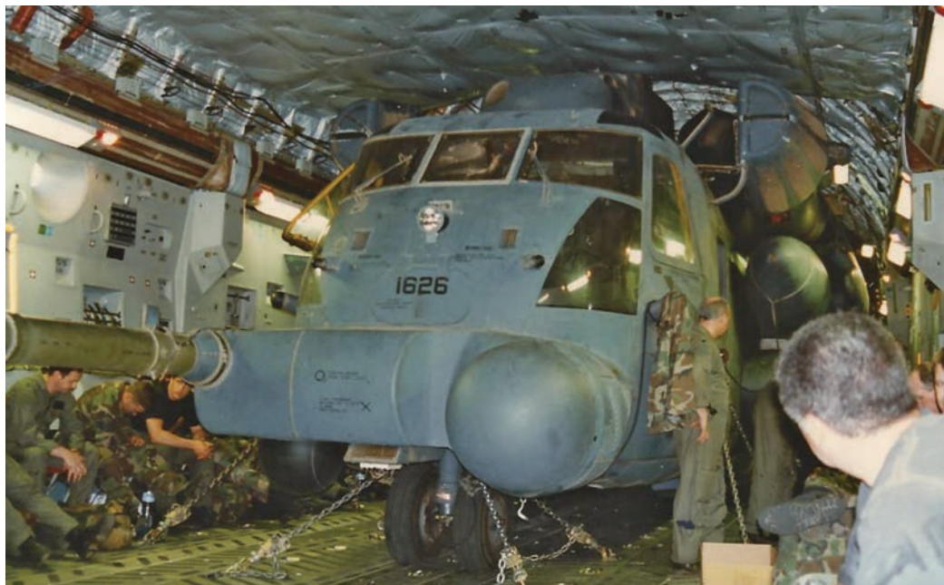
The skills for rapid disassembly and rebuild of MH-53s were honed in the months prior to Eagle Claw/Desert One when Pave Lows assigned to the 1550 ATTW conducting FOT&E at Kirtland AFB. A pair of HH-53Hs (the rescue designation for the Pave Low IIIs) were, in fact, prepared for shipment to provide a rescue force to cover the exfil after recovery of the US hostages in Iran. The machines, maintainers, and crews were enroute in C-5A transport when the Desert One crash occurred. (Photo courtesy of CMSgt (Ret) Frank Dailey)
