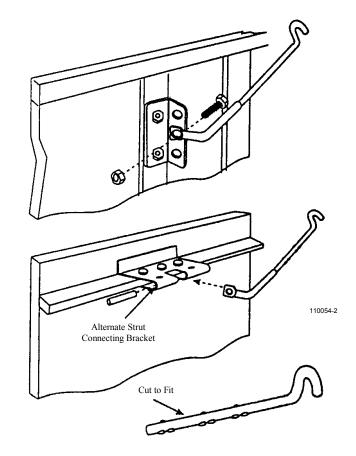
Note: Door Bracket Mount or Strut Mount - If rod bottoms in cushion tube, cut rod to allow for proper function of this assembly.
