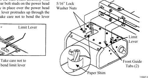
STEP 5: The power head drive unit should be move forward until all play between the gears has been eliminated, but no additional force should be used that could cause pressure on the motor (power head unit) drive gear. Tighten the two 5/16" lock washer nuts on top of the power head drive unit that were loosened in Step 2 above.
