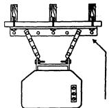
For finished ceilings, or if structural beams are out of position for mounting use a third mounting angle (not included) making sure it is securely mounted to beams.
