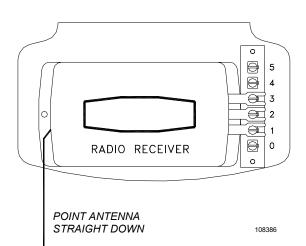
the car. If the distance is still inadequate, try bending the Antenna Wire to a different angle. If the distance is still inadequate, replace the Battery with a standard 9-Volt "transistor radio" Battery (NEED 1604). The Battery is located in the front compartment next to the Coding Switches.
