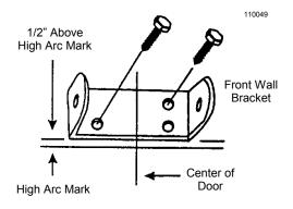
**STEP 3** — Raise the Opener and rest the Power Unit on a ladder or other sturdy support. Open the door the full open position. Allow 2" of space between the Tee Rail and the top section of the door (as shown in the illustration, below on the right).
