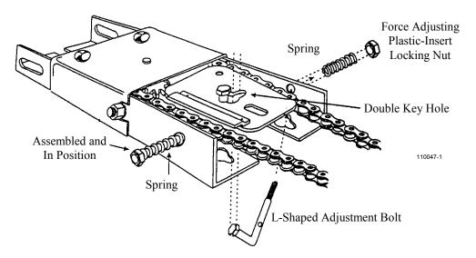
hole. Slide the spring over the bolt and attach load adjusting nut. Tighten until the tip of the bolt extends 3/16" outside the nut. Repeat above for the other side.
