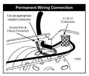
indicate this.) The Opener must be permanently wired with a proper ground connection according to all applicable local, state, and federal building and electrical codes. Run a three (3) conductor (minimum #14, copper
