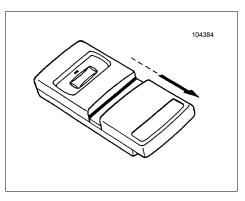
**RECEIVER:** The Receiver Coding Switches can be accessed by removing the small door from the back of the Receiver using a small screwdriver or knife.
