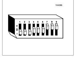
**CODING BLOCK:** Transmitter and Receiver Coding Switches are contained in identical Coding Blocks, consisting of nine small switches, labeled 1 - 9, each of which can be set in any of three positions, labeled +, 0, -
